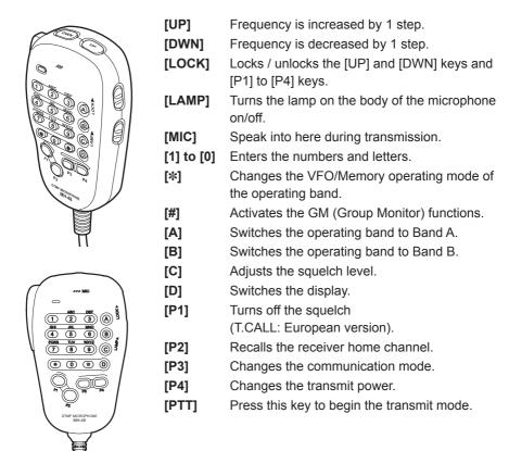
Tip — Preferred functions can be assigned to buttons [P1] to [P4]. Select using the [CONFIG]→[10 MIC PROGRAM KEY] in the set-up menu.
