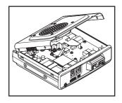
**6** Unplug the speaker cables extending from the top cover from the socket of the board inside the main body first before removing the cover
