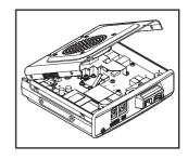
**6** Unplug the speaker cables extending from the top cover to the connector on the board inside the main body first before removing the cover
