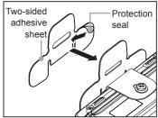
4 Peel off the other protection seal from the underside of the two-sided adhesive sheet pasted onto the bracket, and then stick the bracket to the installation location
