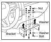
**4** Fasten the main body to the bracket, using the provided flange bolts, as shown in the drawing
