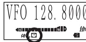
Just press and hold in the **(PWR)** switch for 3 seconds to turn the transceiver back on after an APO shutdown, as usual.
