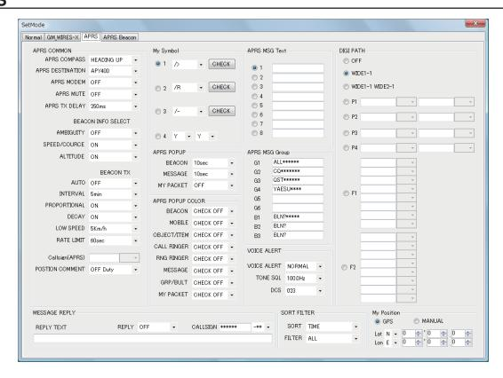
To change the setting of each item in the window, Click the [▼] icon to show the dropdown settings list, and then click the desired selection from the list. Enter the APRS MSG information by placing the curser in the appropriate box and typing the desired data.
