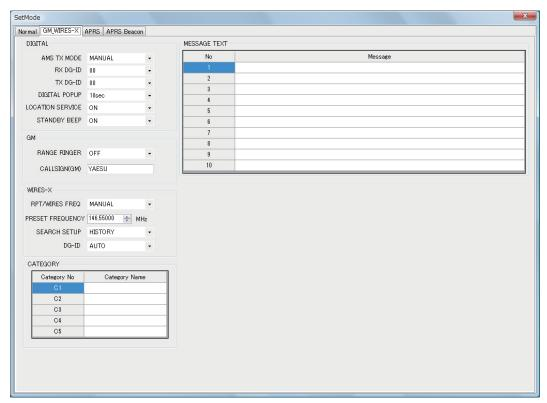
To change the setting of each item in the window, Click the [▼] icon to show the dropdown settings list, and then click the desired selection from the list. Enter the "CATEGORY" and "MESSAGE TEXT" information by placing the curser in the appropriate box and typing the desired data. Refer to the FTM-400XDR/XDE/DR/DE operating manual for the details of each function.
