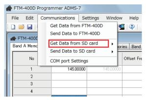
Insert the SD Card with the saved data from FTM-400XDR/XDE/DR/DE to the computer.
