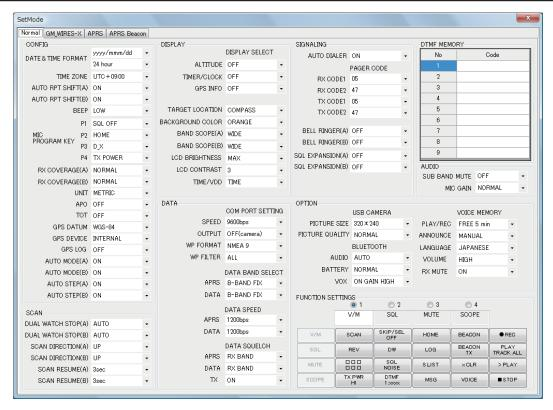
To change the setting of each item in the window, Click the  $[\P]$  icon to show the dropdown settings list, and then click the desired selection in the list. Enter the DTMF MEMORY Codes by placing the curser in the appropriate box and typing the desired data.
