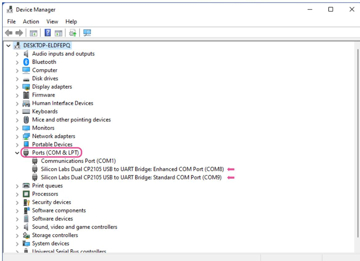
The SCU-17 or an compatible transceiver contain two virtual COM ports, an **Enhanced COM Port** and a **Standard COM Port**. These ports offer the following functions:
