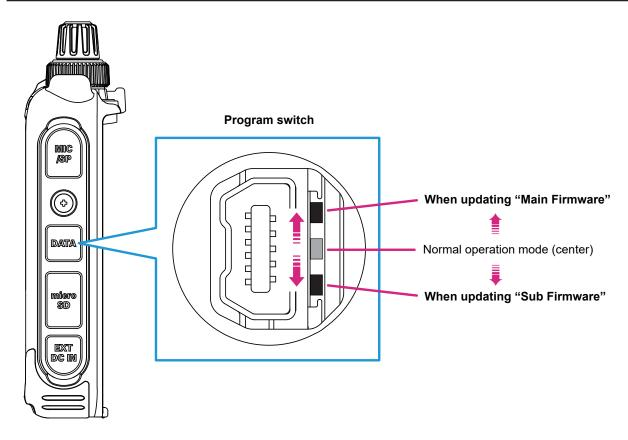
7. Use the supplied cable to connect the FT5DR/DE DATA jack to the computer.
