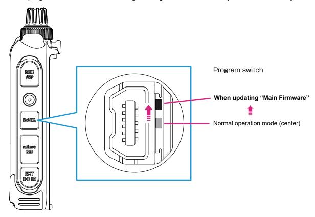
4. Use the supplied USB cable to connect the FT5DR/DE DATA jack to the computer.
