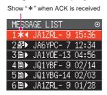
APRS MESSAGE LIST screen (display when an acknowledgment is received)
