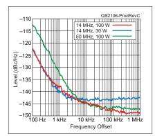
Figure C — The spectral display of the Yaesu FTDx10 transmitter output during phase-noise testing. Power output is 100 W on the 14 MHz band (red trace), 30 W on the 14 MHz band (blue trace), and 100 W on the 50 MHz band (green trace). The carrier, off the left edge of the plot, is not shown. This plot shows phase noise 100 Hz to 1 MHz from the carrier. The reference level is -110 dBc/Hz, and the vertical scale is 5 dB per division.
