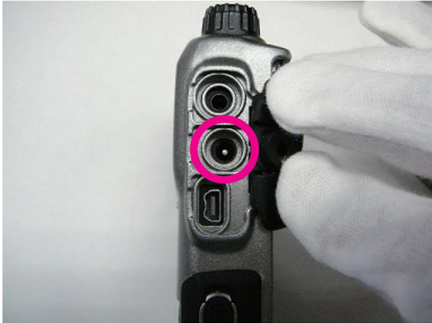
Connect the AC adapter to a wall outlet and then insert the plug to the FT1DR/DE EXT DC IN terminal.
