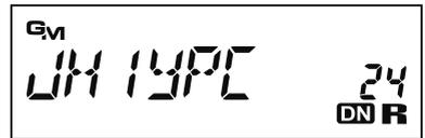
3. Press and hold the [D/A(GM)] key for one second to disable the GM function and return to the frequency screen.
