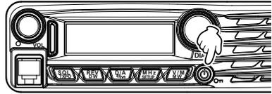
You can compose any desired Opening Message (up to 8 characters) via Setup Menu Item “**OPEN MSG 26**” see 44 for details.
