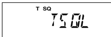
“T SQ” is displayed on the screen. Now the squelch opens only when receiving tone signals of the set frequency.
