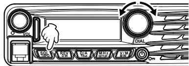
**Note:** A special “RF Squelch” feature is provided on this radio. This feature allows setting the squelch so that only signals exceeding a certain S-meter level will open the squelch. For details, refer to the Advanced Manual (download from the Yaesu website).
