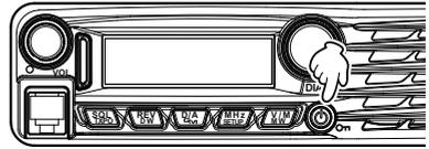
To select which keys are locked, use the Setup Menu Item "**LOCK 22**" see 44 for details.
