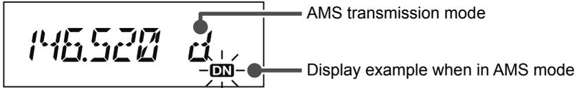
To operate in fixed communication mode, press **[D/A(GM)]** key to switch the communication mode.
