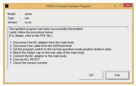
11. Disconnect the AC adapter from the transceiver.
