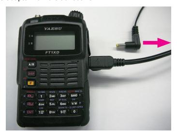
12. Disconnect the cable from the DATA terminal and the computer.
