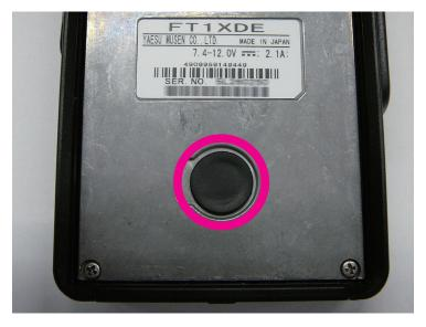
Do not forget to move the program switch at the back of the main body to the normal operating mode position (downward) and then cover up the switch with the rubber cap.
