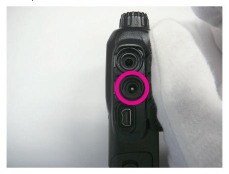
Connect the AC adapter to a wall outlet and then insert the plug to the FT1XDR/DE EXT DC IN terminal.
