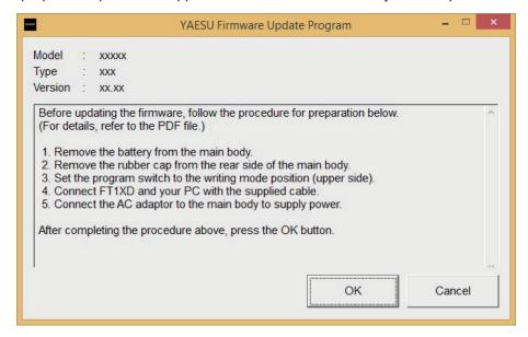
Remove the battery and AC adapter
