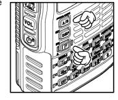
Each time (A/B) is pressed, the operating content displayed on the LCD screen is changed.
