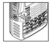
2 Open the microSD cover on the side of the transceiver.
