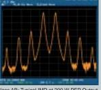
Class A: Ultra-Low TX IMD (PO: 100 W Version) Class AB: Typical IMD at 200 W PEP Output
