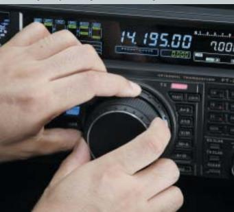
• Just as on the FT DX 9000, the most important switches for operational control are arrayed around the Main Tuning Knob, making the FT-2000 and ergonomic delight. Included are memory control, narrow filter selection, QMB (Quick Memory Bank) keys, and VFO selection and command keys surrounding the knob, with operating mode selection in the next row to the left.
