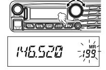
Within five seconds of pressing the [V/M(MW)] key, use the DIAL knob to select the desired memory into which you wish to store the frequency.
