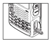
3 Insert the microSD memory card into the card slot until you hear a click. (as shown in the figure at the right).
