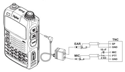
After TNC is connected, set the level of output to TNC by adjusting the sound volume level of your transceiver.
