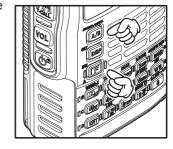
Each time  $^{\text{MONO/DUAL}}$  is pressed, the operating content displayed on the LCD screen is changed.
