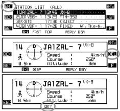
The **FTM-350** Series transceiver enables you to store up to 100 stations into the "Station" list.
