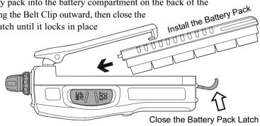
on the bottom of the radio, then slide the battery downward and out from the radio while tilting the Belt Clip out of the way.
