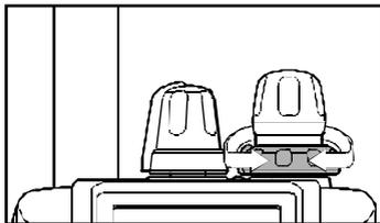
Adjust the **SQL** control just to the point where the noise is silenced and the Green LED is extinguished. If the **SQL** control is set further clockwise, sensitivity to weak signals will be reduced. Now, whenever a signal reaches the receiver that is strong enough to open the squelch, the indicator will glow green.
