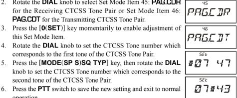
knob to set the CTCSS Tone number which corresponds to the second tone of the CTCSS Tone Pair 6. Press the **PTT** switch to save the new setting and exit to normal
