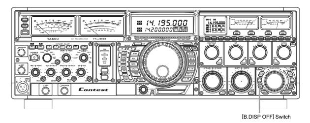
To do this, press the [**B.DISP OFF**] switch, found at the lower left side of the [**CLAR/VFO-B**] knob.
