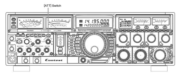
Rotate the **[ATT]** switch to set the desired attenuation level, per the chart below.
