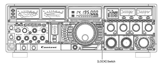
To lock out the [Main Tuning Dial] knob just press the [LOCK] switch that is located to the right of the [Main Tuning Dial] knob. To unlock the [Main Tuning Dial] knob setting, and restore normal tuning, just press the [LOCK] switch once more.
