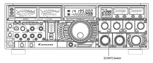
Press and hold the **[CONT]** switch for 2 seconds to activate the Audio Peak Filter (APF) circuit. The LED inside the **[CONT]** switch will blink umber for 3 seconds, then replaces to continuous glow. The APF is an automatic circuit, and there is no adjustment knob for the APF.
