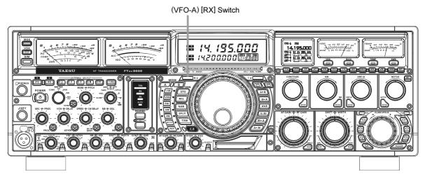
Press the VFO-A band's [RX] LED/switch.
