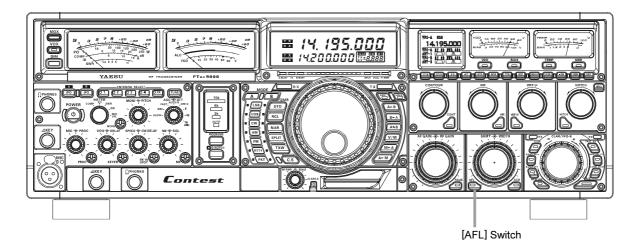
Press the **[AFL]** switch to turn on the Audio Limiter. The imbedded LED in the button will glow red. To disable the Audio limiter, press the **[AFL]** switch once more; the imbedded LED will turn off.
