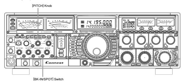
For everyday operation, the (CW) [PITCH] control allows you to set the center of the receiver passband, as well as the offset pitch of your CW carrier signal, to the tone pitch you prefer to listen to.
