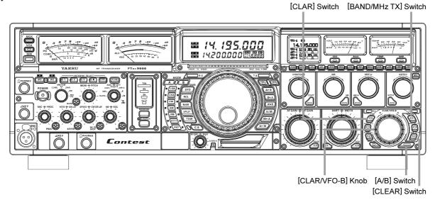
Press the [CLAR] switch. The Red LED imbedded in the switch will light up, and "CLAR" will appear in the display. The [CLAR/VFO-B] knob will now be enabled for offset tuning of the transmitter.
