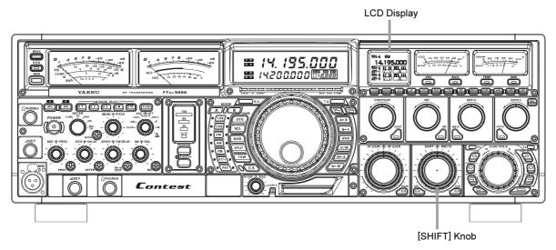
Rotate the **[SHIFT]** control to the left or right to reduce the interference.
