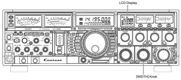
Rotate the **[WIDTH]** knob to adjust the bandwidth. Counter-clockwise rotation reduces the bandwidth, while clockwise rotation increases the bandwidth.
