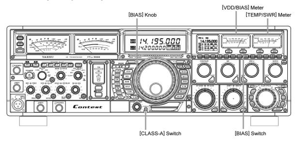
To engage Class-A operation, press the [CLASS-A] switch. The imbedded Red LED will light up, confirming that Class-A operation has been selected.
