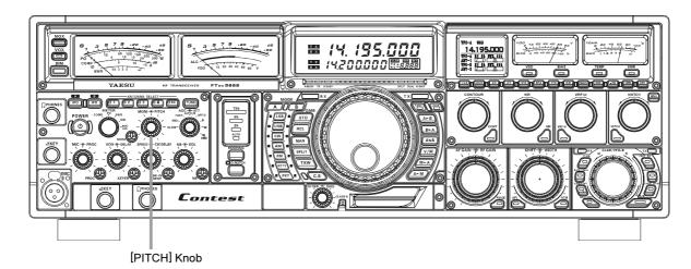
Rotation of the front panel's [PITCH] control will allow adjustment of the center frequency of the receiver passband, as well as the pitch of your offset CW carrier, to the tone you prefer. The tone may be varied between 300 Hz and 1050 Hz, in 50 Hz steps.
