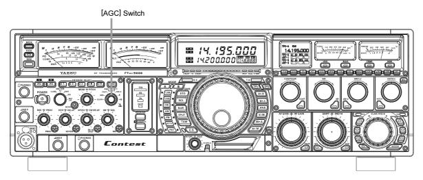
Rotate the [**AGC**] switch to select the desired receiverrecovery time constant. For most operation, we recommend the "AUTO" mode.
