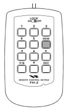
3. Press any of the keys numbered [1] through [5] to select that memory storage register. If you do not press the PTT key (see next step) within five seconds, the memory storage process will be cancelled.
