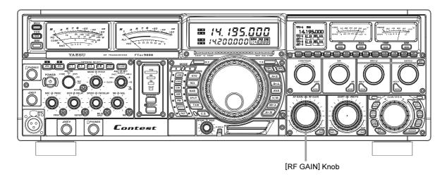
The [**RF GAIN**] control should, initially, be rotated to the fully clockwise position. This is the point of maximum sensitivity, and counter-clockwise rotation will gradually reduce the system gain.
