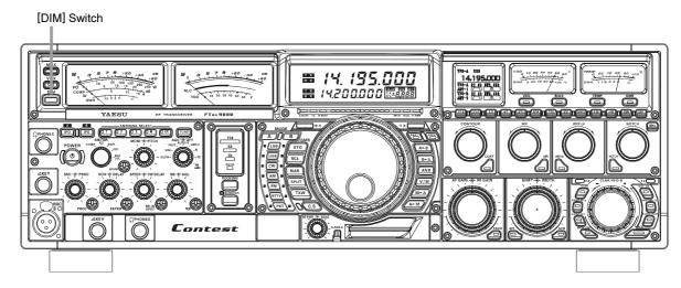
To reduce the illumination level, press the **[DIM]** switch, located to the left of the leftmost analog meter. To restore full brightness, press the **[DIM]** switch once more.
