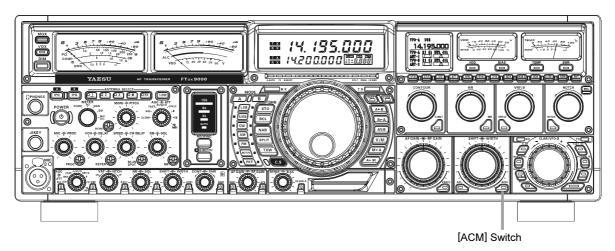
To activate the Adjacent Channel Monitor, press the **[ACM]** switch. The LED imbedded in the switch will glow Red.
