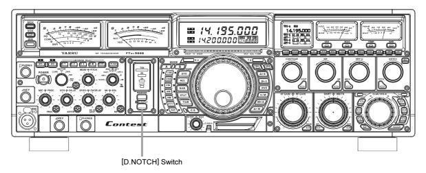
Press the [**D.NOTCH**] switch to engage the Digital Notch filter. The LED imbedded in the switch will glow Red, to confirm that the DNF circuit is engaged.
