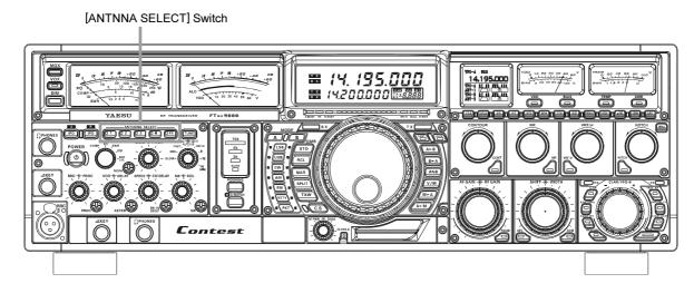
Selection of the desired TX/RX antenna is accomplished by pressing the appropriate  $[1] \sim [4]$  Antenna Selection switch on the front panel.
