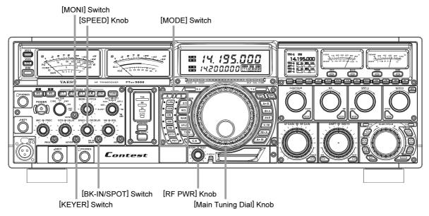
1. Press the [CW] mode switch to engage CW operation. ADVICE
