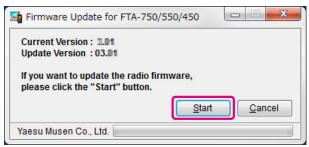
f) Confirm which current version firmware is installed in the transceiver.
