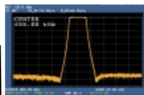
10-pole Collins® Mechanical SSB Filter Passband Response
