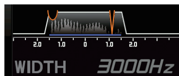
IF DSP Operating Status Display
